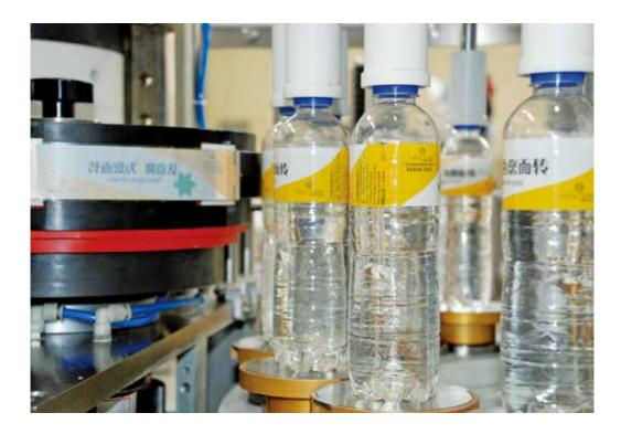
difficult for the speed to match the bottle model ideally. It is easy to pull the label to make it stretched or loosened and the label's misplaced deviation is far more that the result of the servo control system structure.
