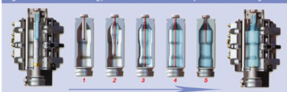
Diagrammatic sketch for the working process within the cabinet of the fully automatic bottle blowing machine
